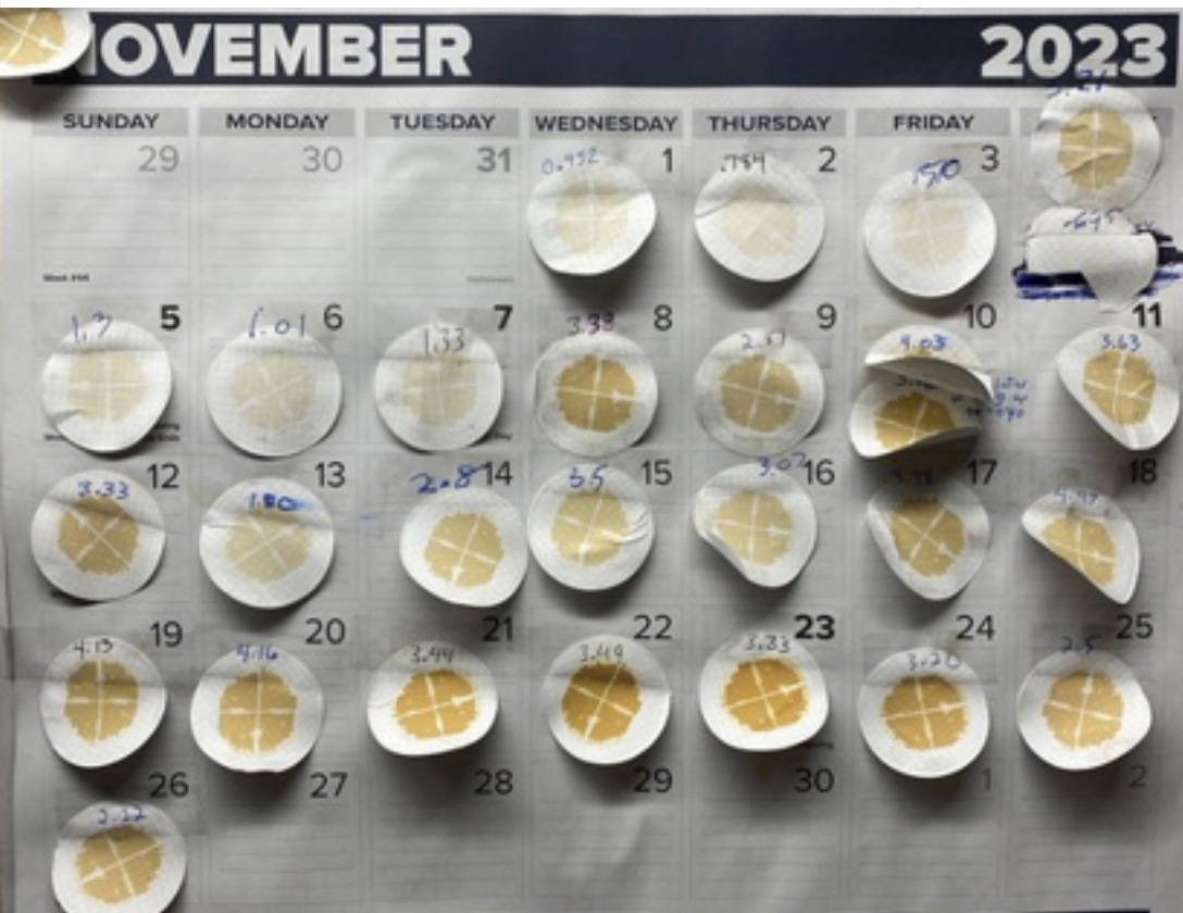
Figure 1: Coupons demonstrating the increase in SDI due to the upstream coagulant upset in November 2023.
